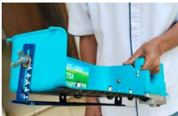
Figure 1. Bantalan pemetikan plucking height pad
